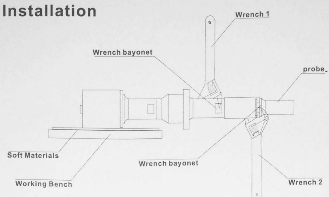
2. Remove the amplitude converter, place the transducer flat on the work table, hold the wrench 1 with the left hand and reverse jam the aluminum alloy part 1 of the transducer, hold the wrench 2 with the right hand and front jam the transformer 2 with the left hand, fasten and fix the transducer with downward force, and clamp the transducer with the right hand and upward force. (soft spacer can be used to protect the surface of the transformer when clamping) as shown in the figure below:
